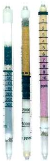
Figure 17: Example of chemical indicator tubes
