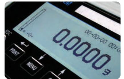
Selectable digital filtering helps minimise effects of vibration and disturbances
