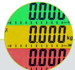
Backlight changes colour during checkweighing
